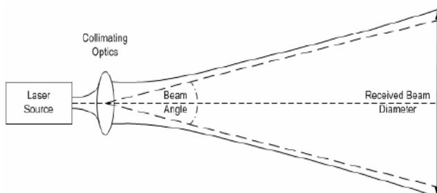
*Fig. 1. Laser beam collimation in long range FSO links.*
